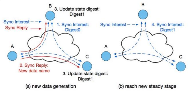
Limitation: cannot directly decode dataset difference from comparing digests
